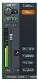
Another difference to the input and playback channels is the **Cue** button instead of Solo. A click on Cue sends the respective Hardware Output's audio to the **Main** Out, or any of the Phones outputs (option *Assign / Cue to* in the Control Room section). With this any hardware output can be controlled and listened to through the monitoring output very conveniently.
